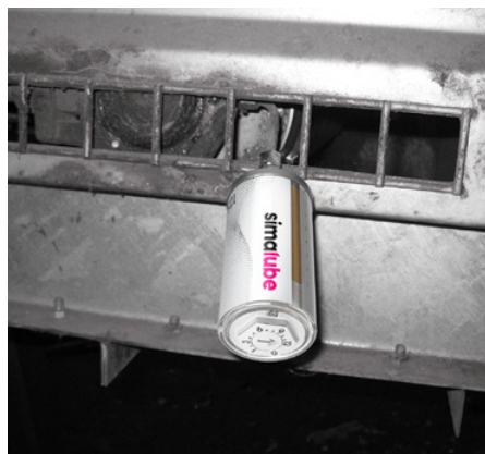
simalube lubricates bearings on a conveyor belt.
