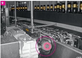
1 Bearing lubrication with **simalube**® 250 ml on an apron conveyor
